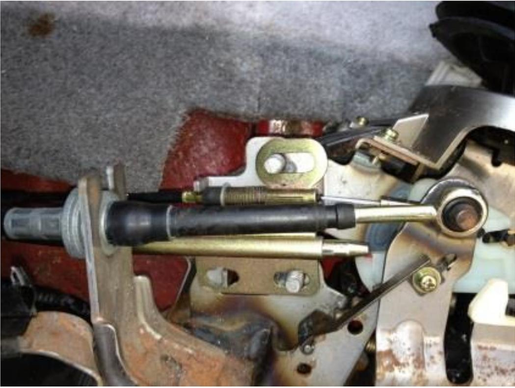
6. These are interchangeable. You need to enlarge the holes for the brake pedal safety switch to mount on the new shifter.
