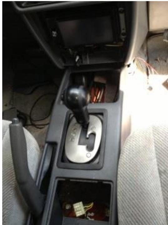
1. Obtain (from a junkyard) a shifter from a 2000-2005 Mitsubishi Eclipse GT (only the GT models, with the V6, have the tiptronic/slap-shift style shifter, wire colors are different from 00'-01' and 02'-05'). Make sure you get as much of the wiring as possible and the rubber grommet that the shift cable goes on.
